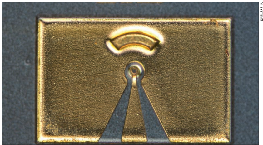
VI Systems' 850 nm quantum-dot VCSELS are suitable for ultra-high-speed data communication.
