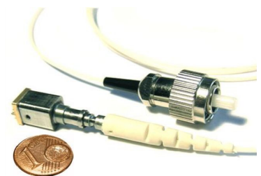
a TO-can sized fiber-coupled 40 Gb/s optical module
